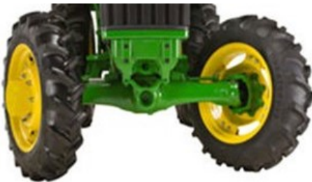
Heavy-duty MFWD front axle on 5E
