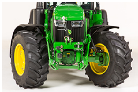
MFWD front axle on 5M with turnable fenders
