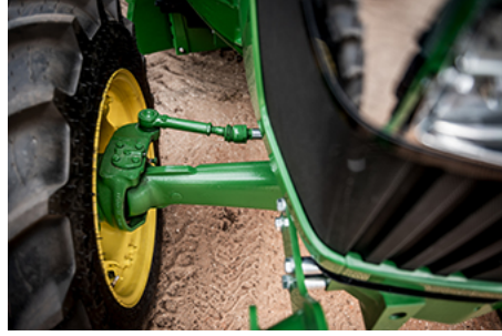
Steering connections are protected by axle shown on 5E 3-Cylinder
