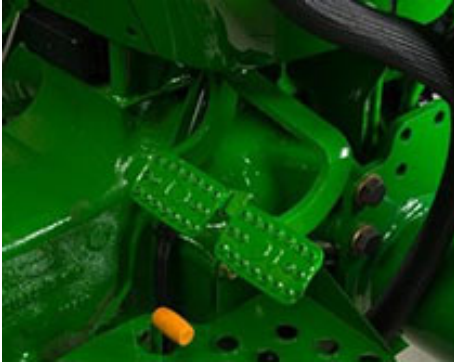
Wet-disc brakes on open operator station (OOS)
