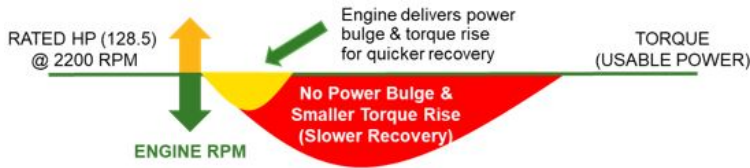
Power bulge and torque curve
